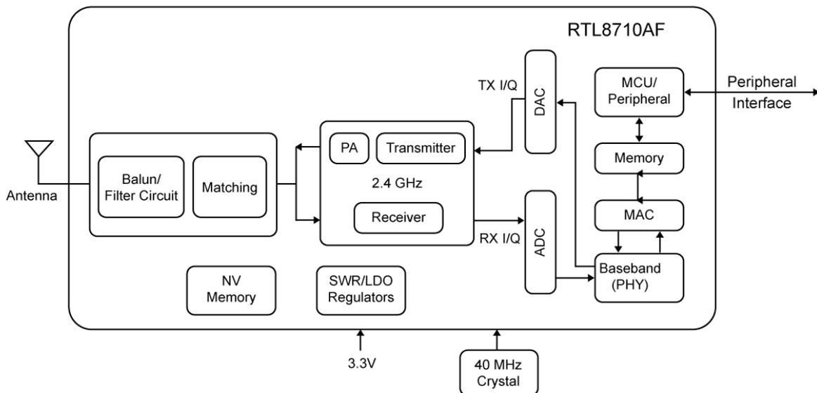
RTL8710AF built-in cache improves system performance and reduces memory requirements. With on board 1MB Flash, PADI IoT stamp can be programmed to run custom firmware that can communicate with external sensors or chipset through various interface ports such as SPI, UART, I2C, PWM and GPIO.
