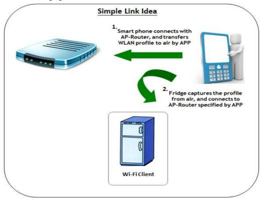
To setup the environment: First, install simple config app on android phone, and second, configure device in log service mode (UART console mode). The detail of application usage and platform setting are introduced in the following subsections.
