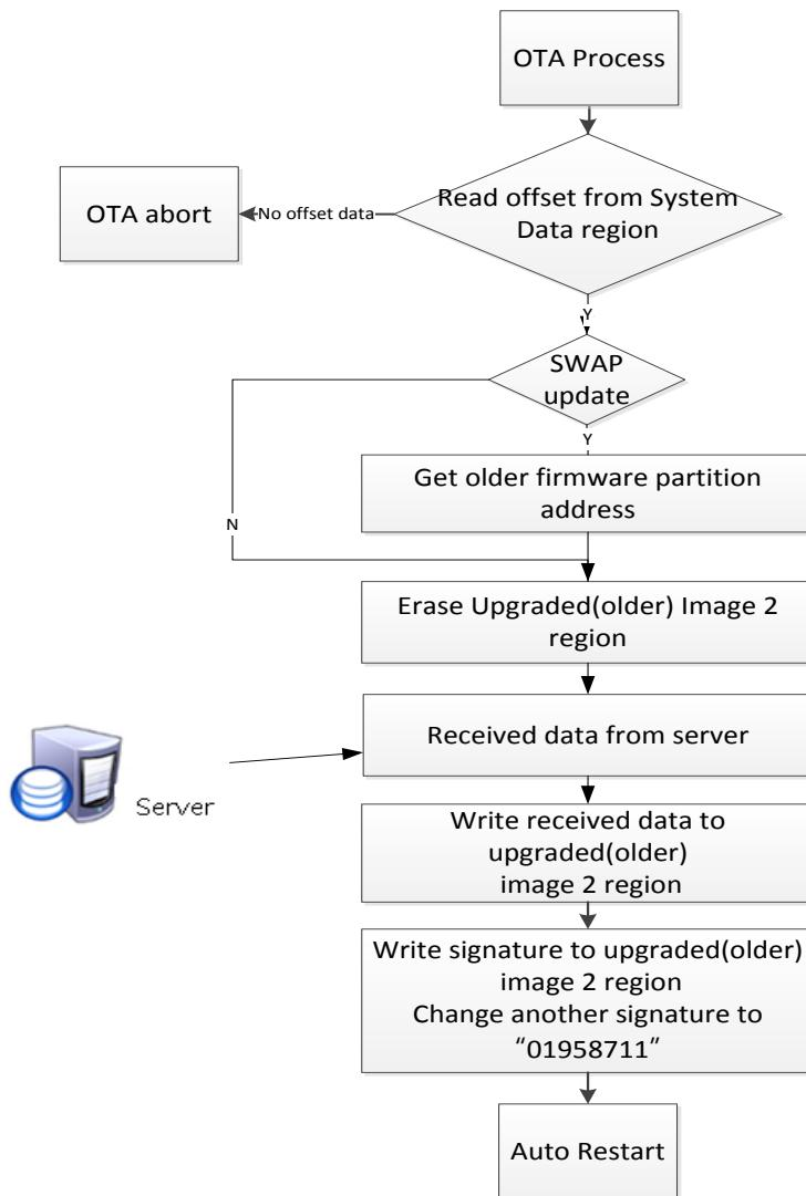
Note: During the step of “Erase Upgraded (Older) Image2 region”, the signature is set to 0xffffffff, which is invalid signature.
